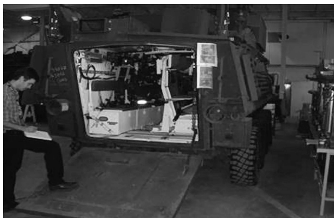
FIGURE 1. Interior view of the Bison command, control, communications, and intelligence mobile command post (Bison C3I MCP).
