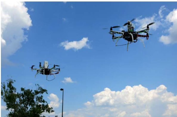
Drone carried on-demand WiFi prototype systems. Photo Credit Yixin Gu,
